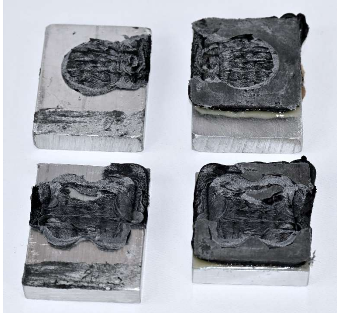
Figure 3.21 Bulk 3D printed ABS/CF failure of tensile test samples.
