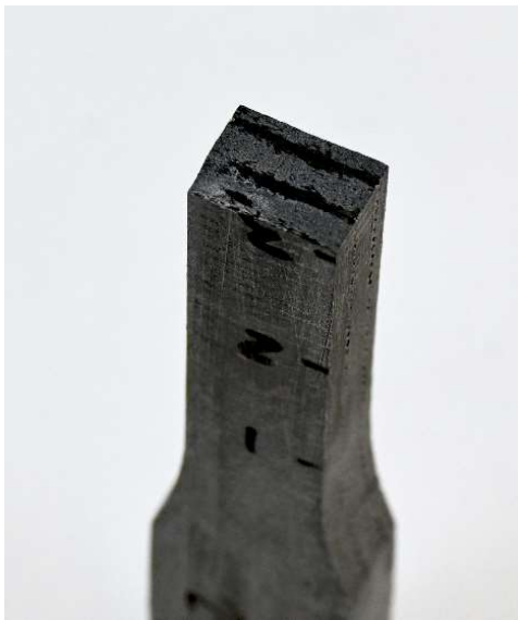
Figure 3.13 Fracture surface of a tensile test bar.
