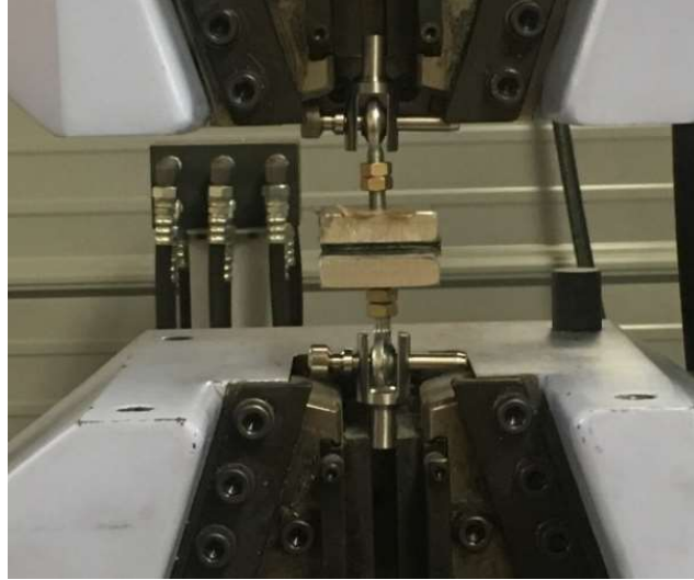
Figure 3.18 Tensile test setup for the mechanical interlocking root.
