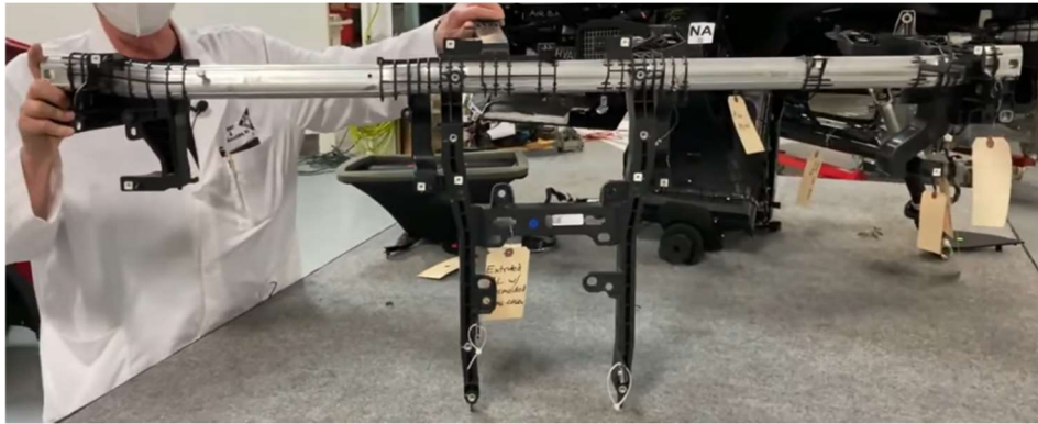
Figure 1.4 A hybrid hydroforming-injection molding metal-polymer component from the Tesla Model Y (Munro Live 2020).
