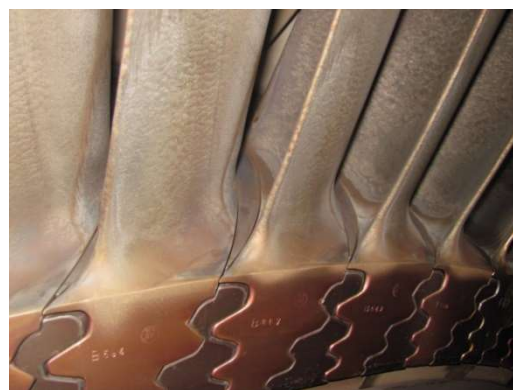
Figure 3.2 Mechanical interlocking features retain gas turbine blades (Combined Cycle Journal, 2012).
