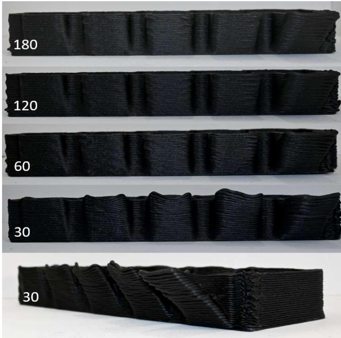
Figure 3.8 Un-anchored overhang test samples with 30, 60, 120, 180 second minimum layer time enforced by pausing at the end of each layer.
